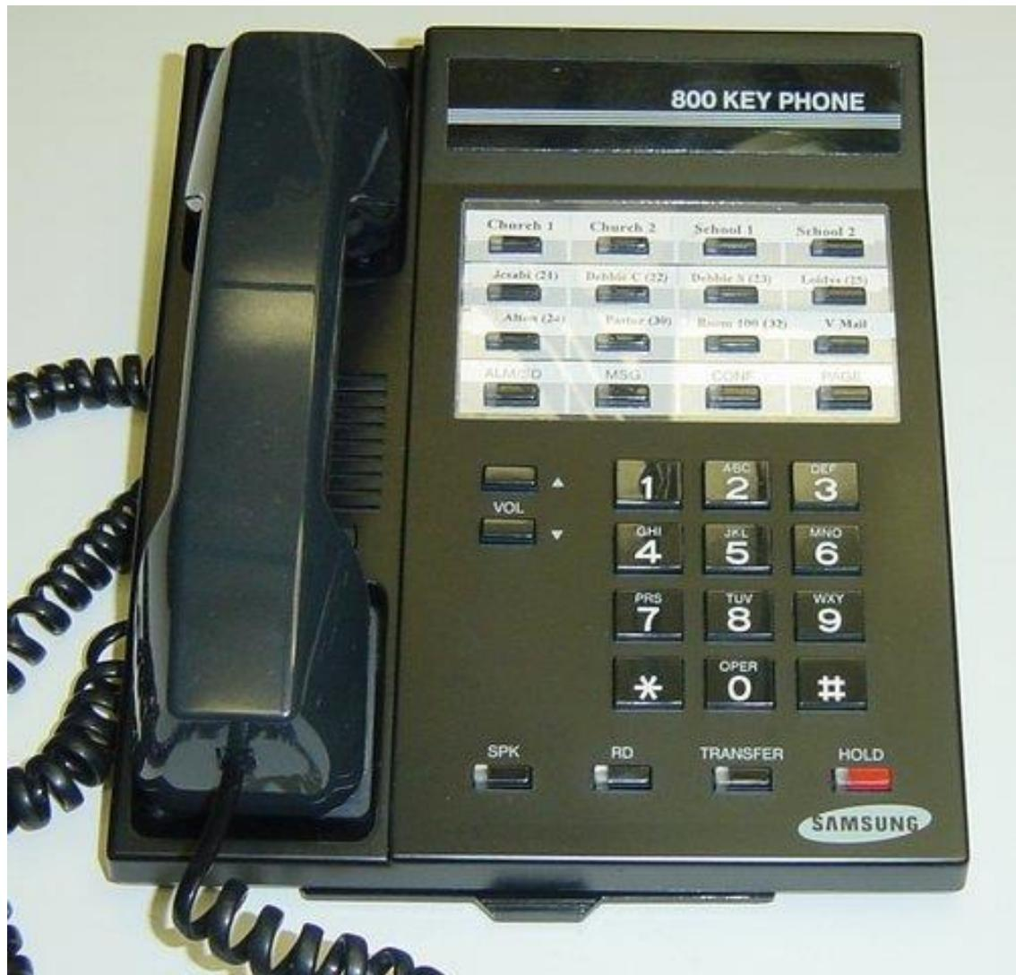
A key system is a multiline telephone **system** typically used in business environments, encompassing **systems** ranging from small **key** telephone **systems** to large-scale private branch exchanges.
