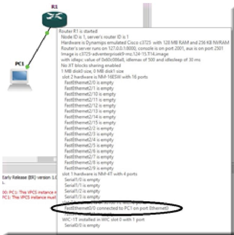
If you can ping the other interface's address, you have successfully configured your VPCS and your gateway router interface. There is still much to do with this router like configuring a static route and or configuring routing protocols, but that is beyond this section.
